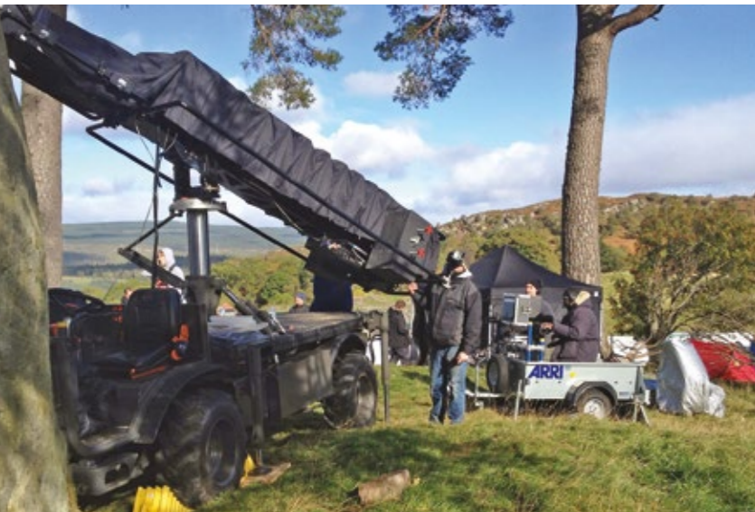
The Taurus vehicle with telescopic crane mounted – Andrei is operating from the trailer behind
